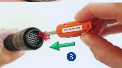
Push the cleaner 1X until it bottoms out for cleaning the endface
