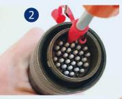
2 Open the cover on the red endcap and insert the cleaner onto the first ferrule.
