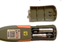
Remove the batteries when the VFL is in storage to prevent battery leaks
