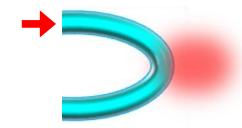
Macrobending is happens when the fiber exceeds the bend radius.
